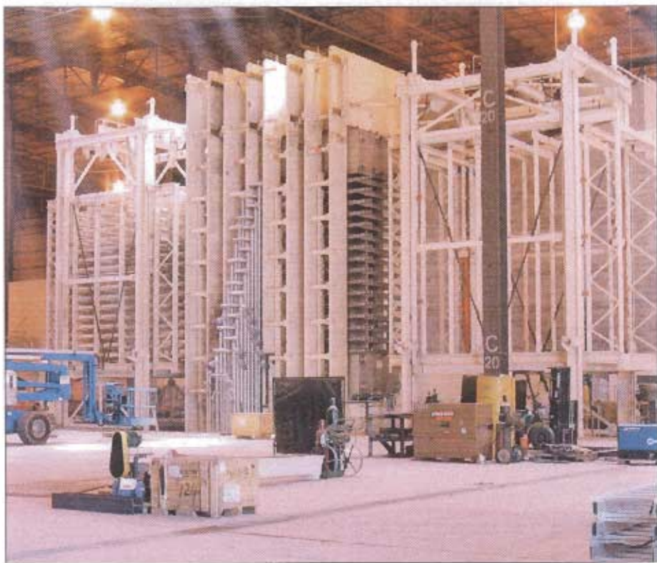
Siempelkamp 16-opening press as it looked three months before startup.
